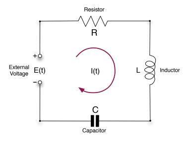
In an RLC-circuit we have a resistor R (ohms), an inductor L (henrys), a capacitor C (farads) and an source of electromotive source E(t) and the following voltage drops:
