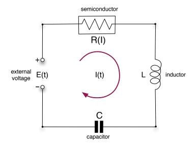
This is an RLC loop, but with the passive resistor of Ohm's Law replaced by an active element which would pump energy into the circuit whenever the amplitude of the current falls below a certain level. In the 1920's this active element was an array of vacuum tubes, now it is a semiconductor device. B. van der Pol assumed the nonlinear resistor to be represented by the nonlinear function  $R(I) = aI^2 - b$  and substituting R(I) for R in (3) the current in the circuit turns out to be modeled by
