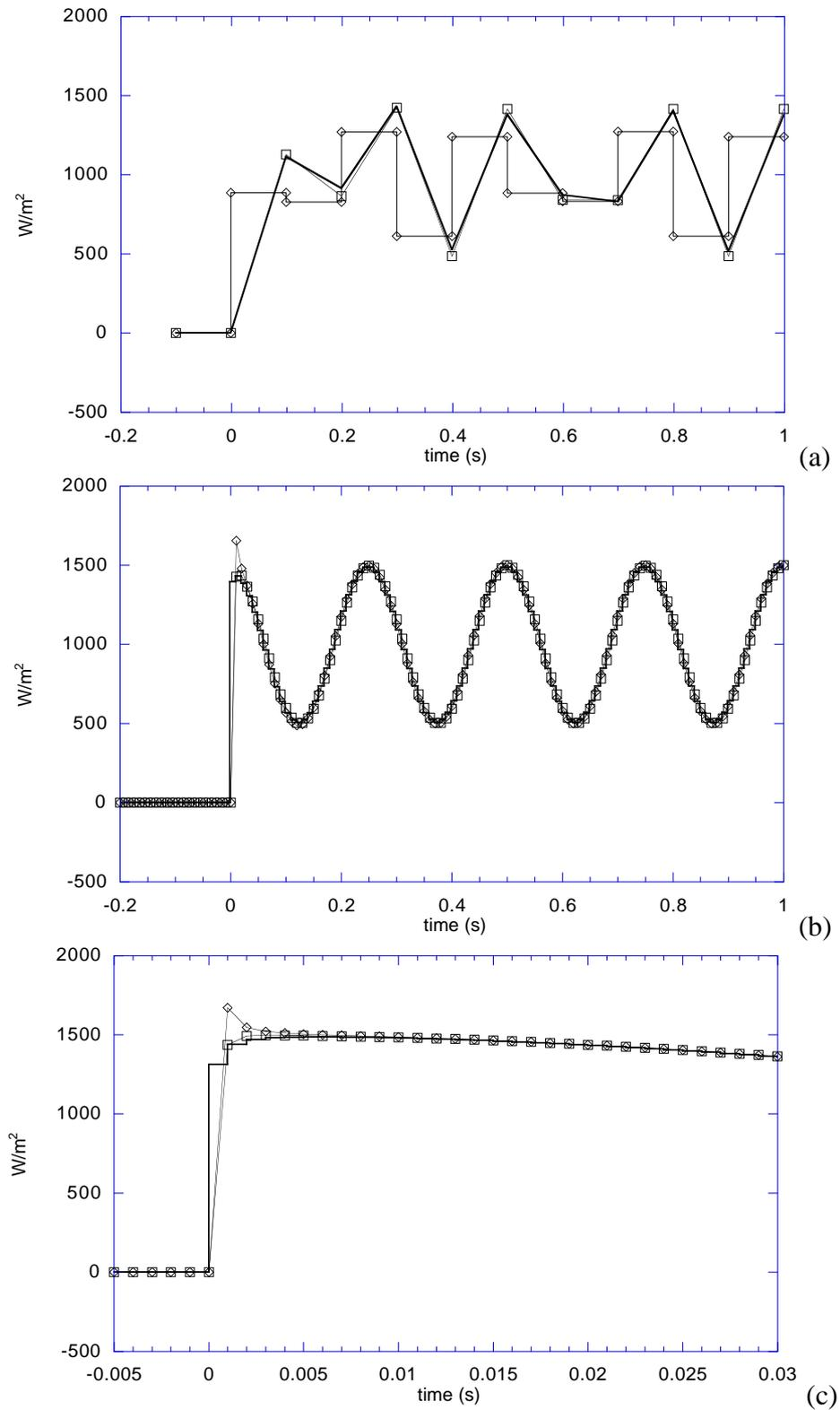
Fig. 7. Oscillating signal reconstruction for double layer configuration (tests 10, 11, 12)
