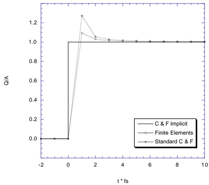
Fig. 4. Single layer heat flux reconstruction (tests 1, 2, 3)
