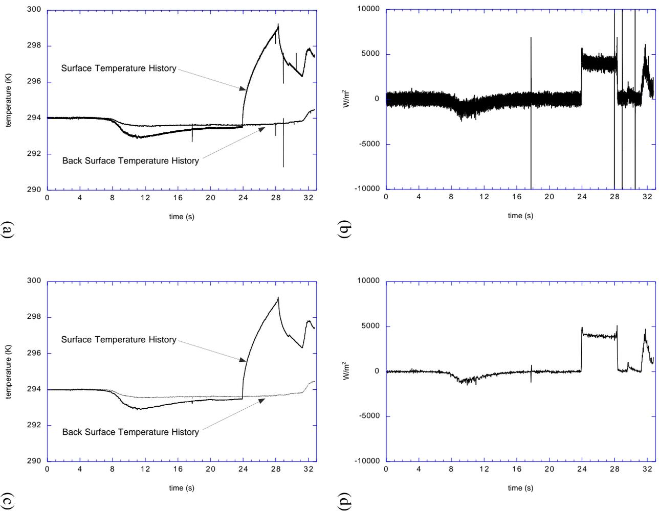
Fig. 10. Single layer thin film surface temperature signal and heat flux computation for test case 15
