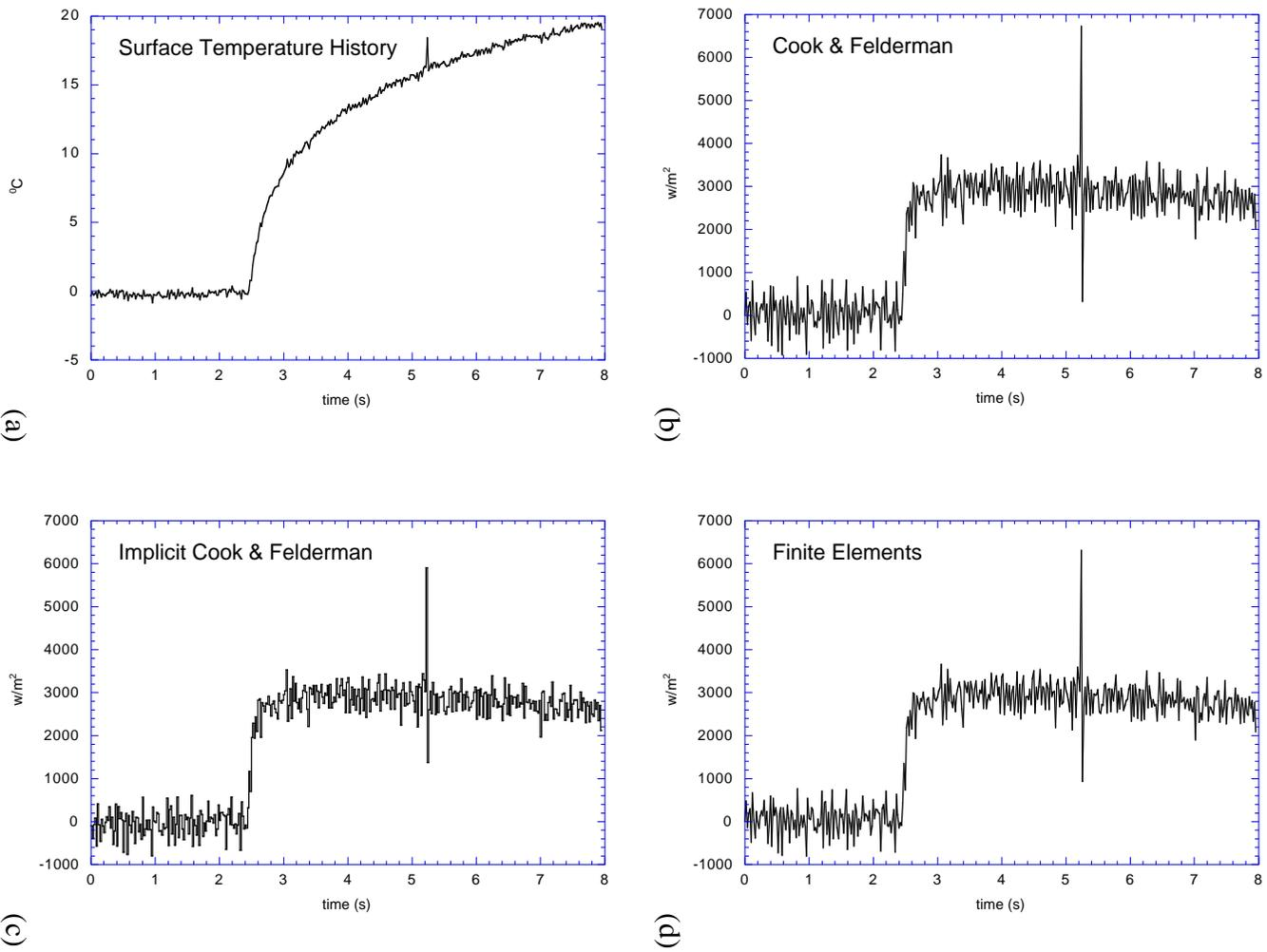
Fig. 8. Double layer thin film surface temperature signal and heat flux computation for test case 13
