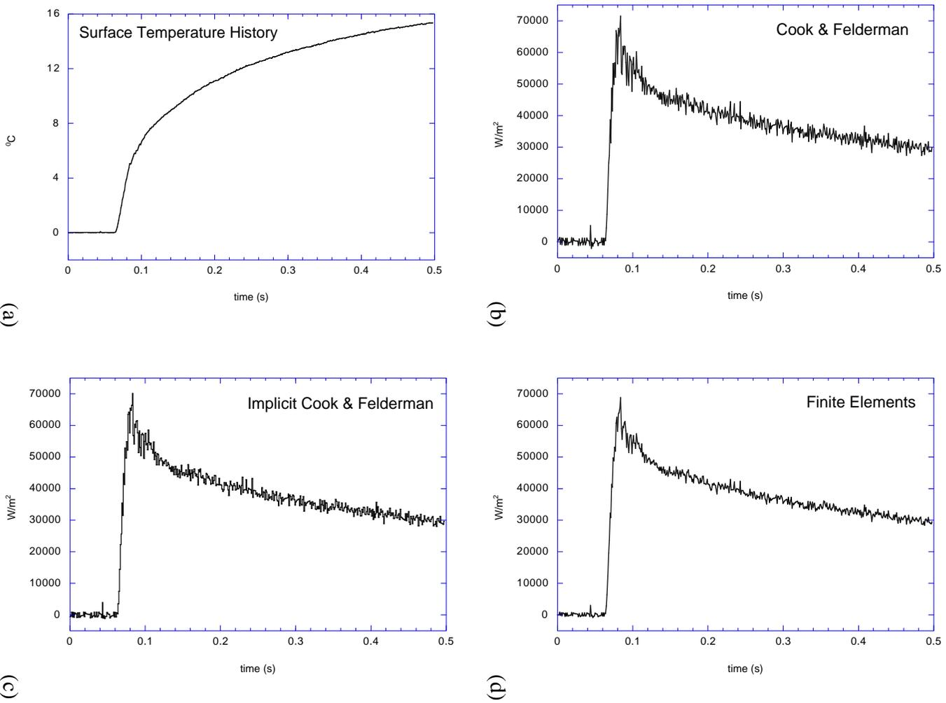
Fig. 9. Single layer thin film surface temperature signal and heat flux computation for test case 14 at Mach 0.7
