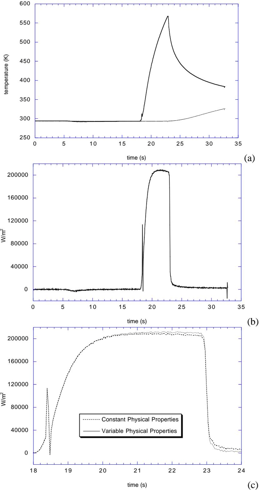
Fig. 11. Single layer thin film surface temperature signal and heat flux computation for test case 16
